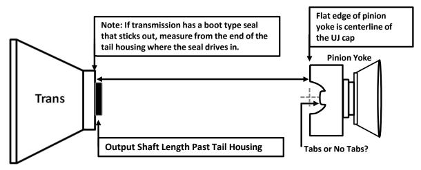
Note: OE Ford 8" and 9" Pinion yokes can use either a 1 1/16 or 1 1/8 cap diameter.
