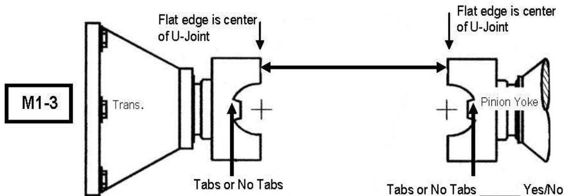
Length from flat edge of yoke to flat of other yoke is same as center to center of UJ cap.
