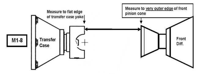
Length from flat edge of transfer case yoke to edge of flange on front differential. Exactly as shown by arrows. Edge to edge only.
