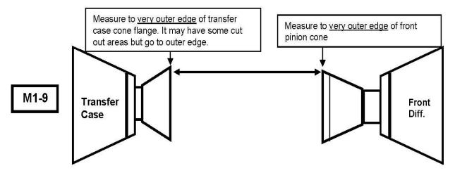
Length from edge of transfer case flange to edge of flange on front differential. Exactly as shown by arrows. Edge to edge only.
