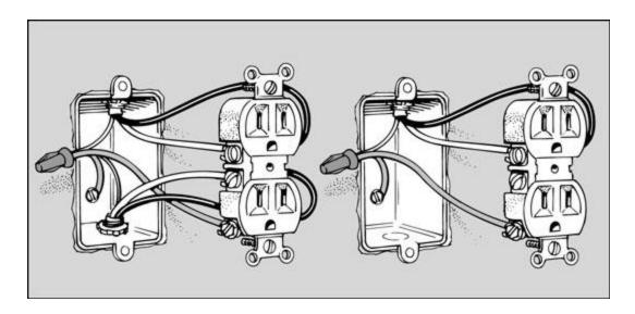
You may also wire the receptacle so that a switch controls the upper outlet and the lower outlet is on, or hot, all the time. In this case, you need to remove the break-off tab connecting the two sets of like-colored terminals on each side of the receptacle. Otherwise, the tab remains intact, and you can see a metal bridge connecting the terminals.
