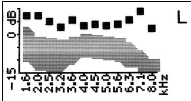
The *DP/TE-Gram graph* displays the absolute values of the signal (emission) as a block plotted at the intersection point of the test frequency (Hz) along the horizontal axis and the amplitude (dB SPL) along the vertical axis.
