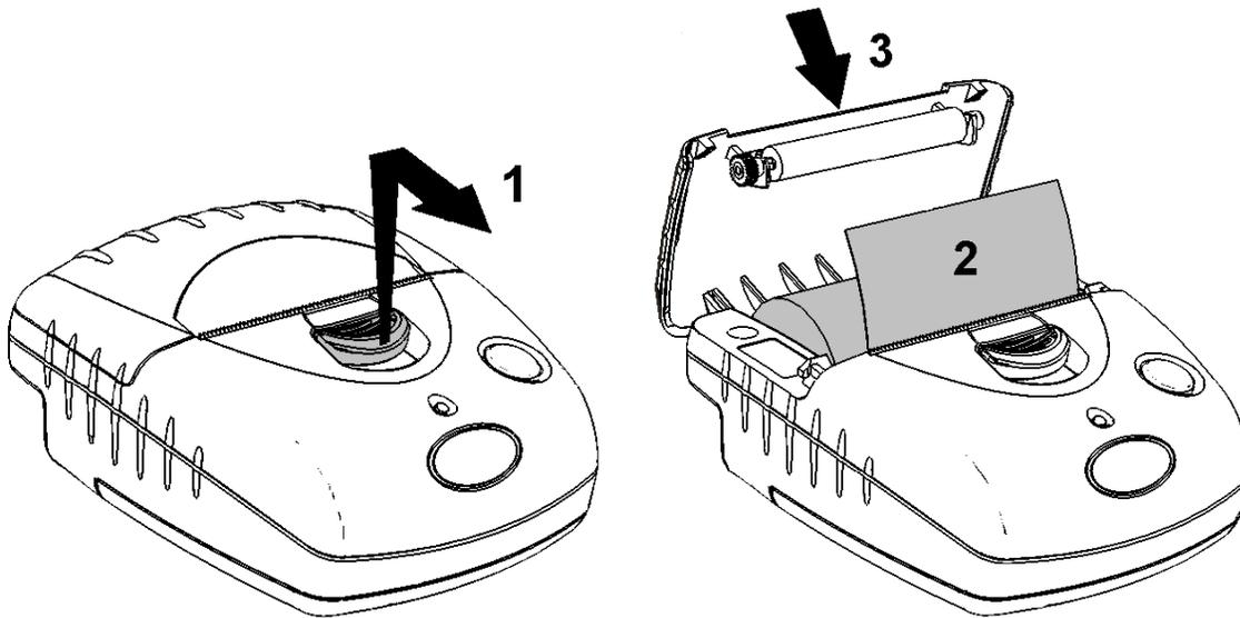
After loading, check that the paper is straight and advances properly. Tear off any excess paper by pulling the paper sharply towards you across the serrated tear bar. In the event of a jam or other paper loading problem, release the lid and straighten the paper before closing again.
