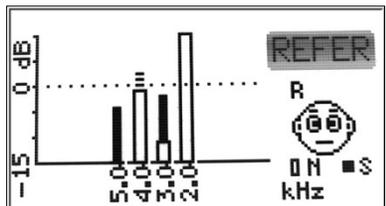
The *Value graph* displays the absolute values of the signal (emission) and noise floor. The noise is represented by an open bar. The signal is represented by a solid bar when it meets the pass criteria and as a dashed bar when it fails to meet the pass criteria for the protocol. When viewing the value graph the user can immediately see if noise was a contributing factor in obtaining a Refer.
