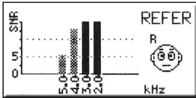
The *SNR graph* shows signal-to-noise ratio (SNR) for each test frequency. SNR is the difference between the measured emission and measured noise floor. The SNR is shown on the vertical axis so the height of each column represents the SNR for that test frequency. For example, if the column goes to the top of the display then the SNR is 15 dB or greater.
