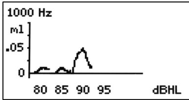
During the measurement of the acoustic reflex the change of the compliance is represented on the instrument display as shown to the left. The zero-line at the bottom of the graph indicates the measured compliance without a test sound. Changes in compliance are shown as deviations from the zero-line. If a Stapedial reflex occurs, the compliance increases and the curve rises. The change in compliance is shown for each intensity level for the stimulus being presented.
