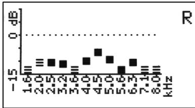
A bright solid block indicates that the SNR is at least 6 dB for DPOAE and 4 dB for TEOAE. A hashed block indicates that the SNR is less than these specified values. Examples are shown in the display to the left.
