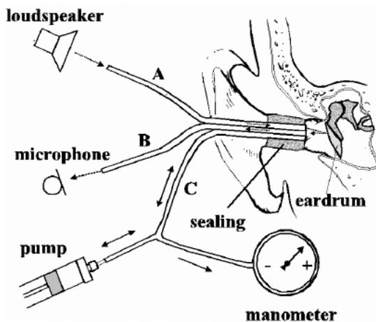
Gradient calculations are reported as the tympanogram width at half of peak compliance expressed in daPa. A "limits" box is available on both the display and printout to aid in diagnosis. Compliance is measured with respect to an equivalent volume of air, with the scientific quantity milliliter (ml). Air pressure is measured in deca-Pascals (daPa).
