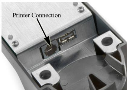
Use the included printer connection cable to connect the cradle to the printer. Connect the appropriate end of the connection cable into the serial data port at the rear of the printer. Connect the opposite end of the data cable into the printer connector on the underside of the cradle.
