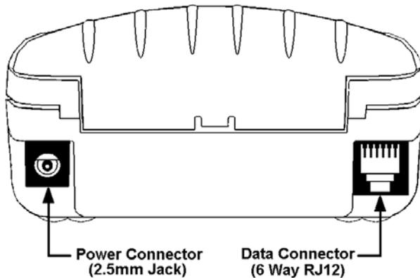
The printer is permanently powered up and ready to print once the power supply is connected to the printer and an outlet. The light on the face of the printer will illuminate solid green when the printer is powered up and ready to print. A flashing green light indicates the printer is not ready (paper low, no paper loaded, lid open, etc...). No light indicates the printer is off.
