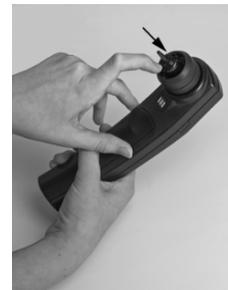
Obtain a replacement probe tip and orient the tip with the arrows on the face of the probe tip directed toward the top of the instrument. The probe tip will only fit on one way; be careful not to force the tip in place. Push the tip directly down onto the probe. Once the probe tip is in place on the probe, push firmly downward on the top of the tabs one at a time until a click is heard. Tug lightly on the probe tip to verify that the tip is securely attached.
