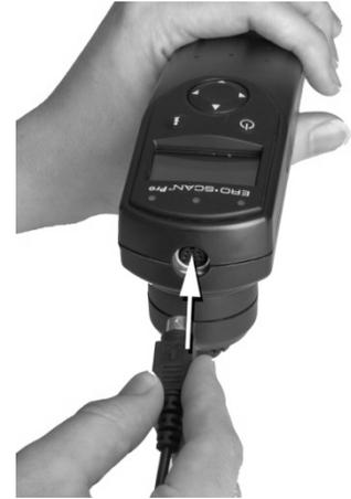
**Note:** Misalignment of the plug and socket when installing the remote probe can cause damage to the pins in the plug and the pin receptacles in the socket. The plug and socket should be visually inspected prior to each installation of the remote probe. If damage is observed, contact your Special Equipment Distributor or Maico Diagnostics.
