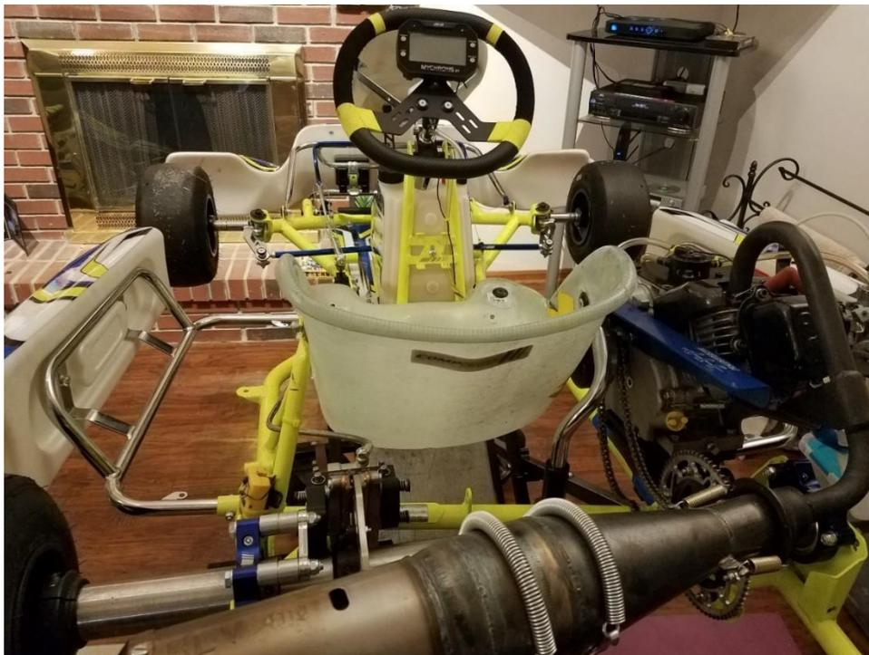
When mounting a seat the first thing you are going to want to do is start by positioning the seat on the kart. To do this you want to seat the seat to be flat with the bottom of the frame rails.
