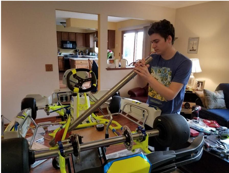
Some karts will come with adjustable seat mounting struts. The COMPKART Covert 4R comes with an adjustable right side seat strut. If the seat struts are fixed, there are a few ways to move them over. One is banging on it with a rubber mallet. However, what I have found is by far the easiest approach is to use a 40mm or 50mm axle. Place the axle in the hole of the seat
