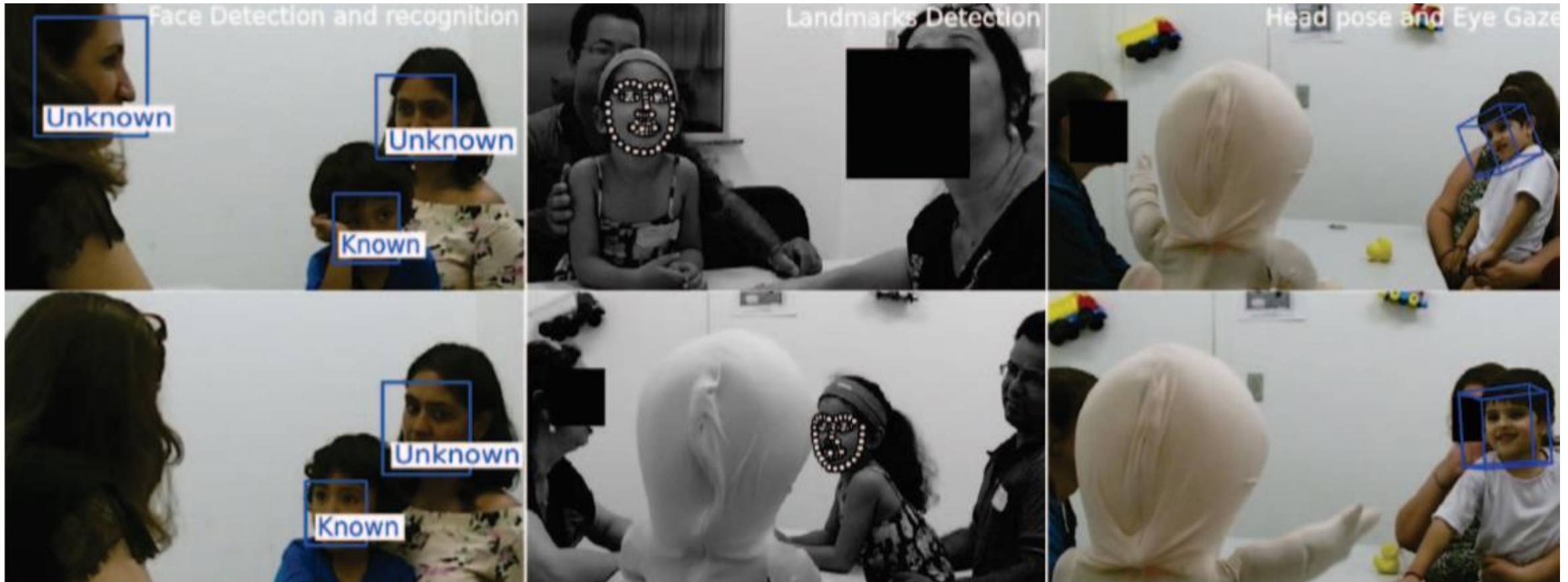
Fig. 15. Performance of the child's face analysis pipeline for the case study. Face detection and recognition, landmarks detection, head pose and eye gaze estimation were executed. Ramirez Duque A. A. et al (2018) [6]
