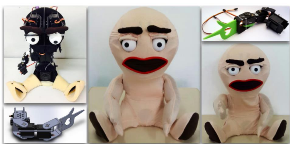
Fig. 7. Physical structure and appearance of the robot ONO. Andrés A. et al (2020) [4]
