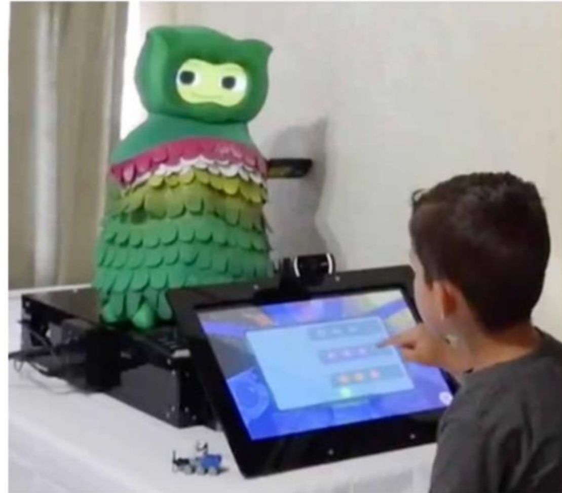
Fig. 16. Long-term, real-world SAR intervention setup. In this month-long, in-home study, child participants with ASD played math games on a tablet, while a socially assistive robot used multimodal data to provide personalized feedback and instruction (37). Jain et al (2019)[7]
