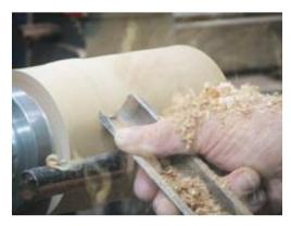
Law #4: The only part of the tool that should be in contact with the wood is that part of the tool that is receiving direct support from the tool rest.
