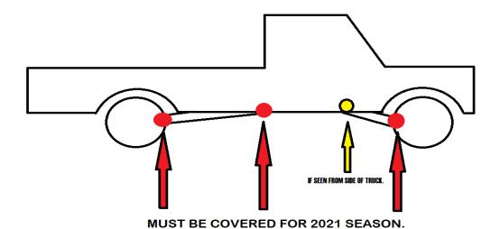
10 B. Minimum of 3 driveshaft loops on rear driveshaft, and as many as practical (minimum of 1) on front driveshaft evenly spaced. Constructed of at least 1/4 inch steel or 3/8 inch aluminum that will safely contain the drive shaft.
