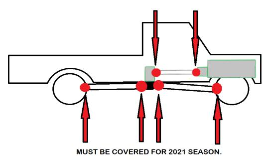
25 B. Minimum of 3 driveshaft loops on rear driveshaft and as many as practical (minimum of 1) on front driveshaft evenly spaced. Constructed of at least 1/4 inch steel or 3/8 inch aluminum that will safely contain the drive shaft.
