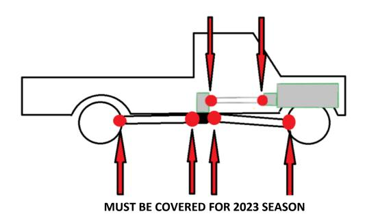
25 B. Minimum of 3 driveshaft loops on rear driveshaft and as many as practical (minimum of 1) on front driveshaft evenly spaced. Constructed of at least 5/16 inch steel or 3/8 inch aluminum that will safely contain the drive shaft.
