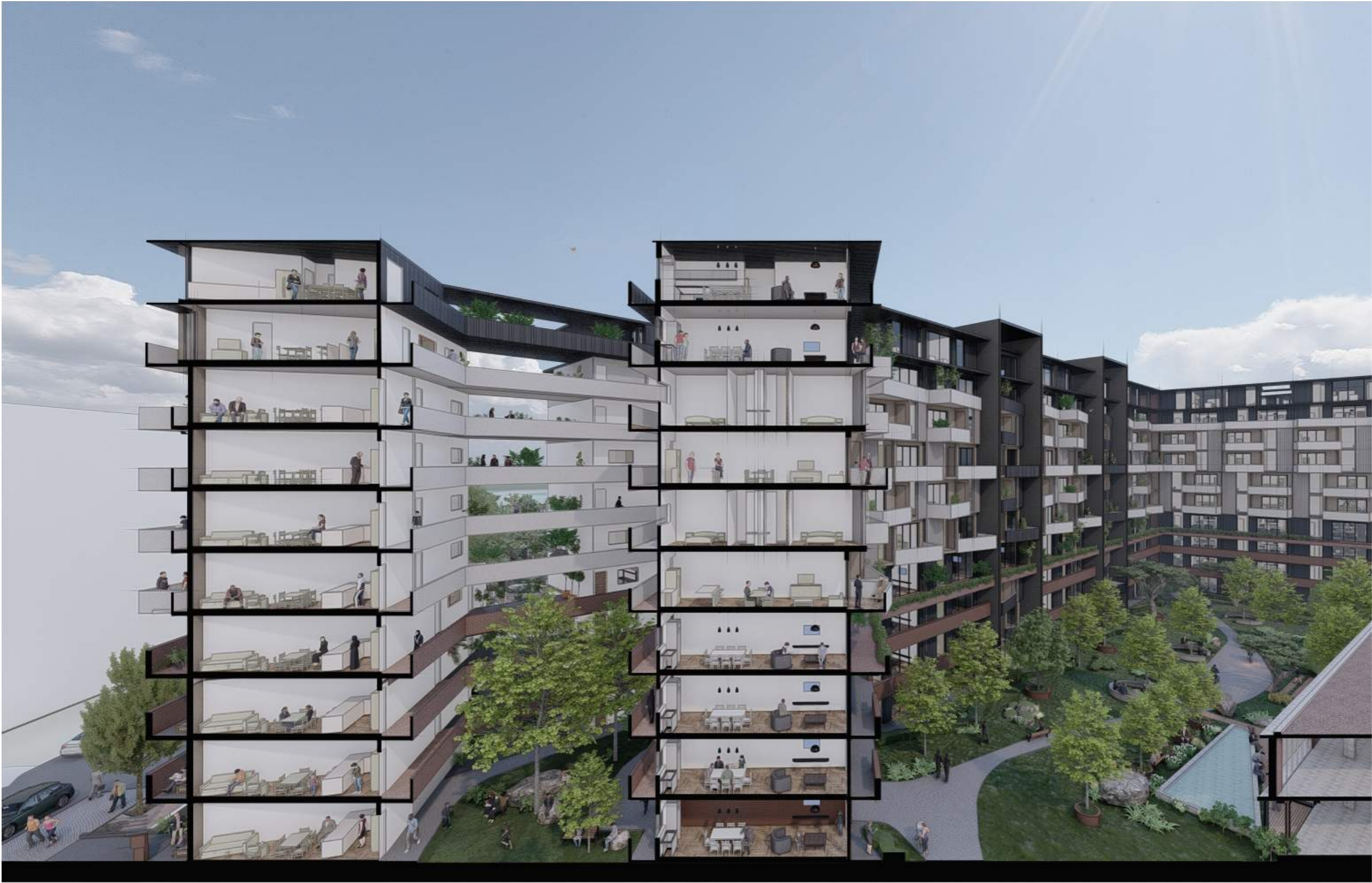
Atrium with Memorial Garden • Creates communal space • Allows building to breathe • Integrates inside with outside • Creates passive cooling & airflow • Creates variety • Invites light into back of living
