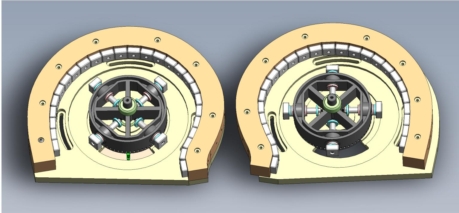
Since magnetic interaction between the two ring-rotor geometries is insignificant, we can simplify analysis by modeling only one
