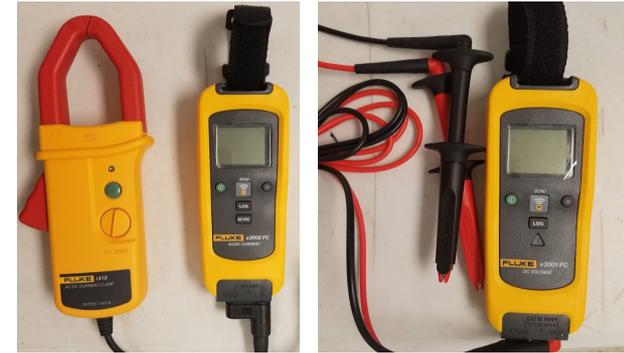
**Voltage Probe: Fluke V3001 FC Wireless DC Voltage Meter**
