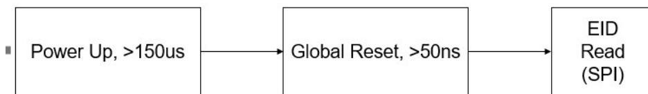
Figure 12 Pre-condition of EID Read
