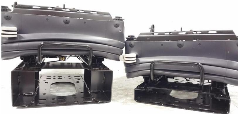
Step 5. Install Quick Connector to new low rider base on same spot ( Use Plastic Tie to install )
