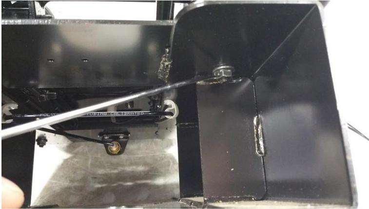
Step 2. Unscrew total 4 bolts. Your bracket will be detached, but still air line has been connected.
