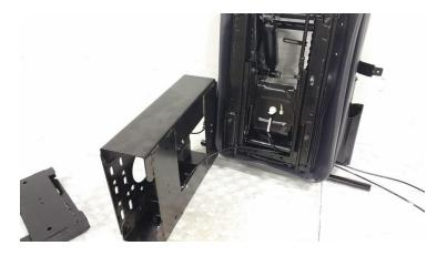
Step 3. Disassemble Quick Connector ( Terminate Two Rivet )
