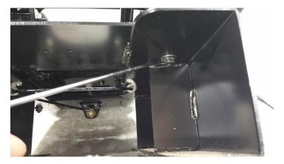
Step 1. Find 4 Bolts from bottom of Bracket (Located between Bracket and Slider)
