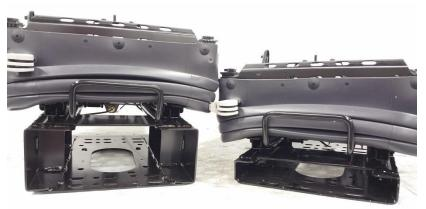
Step 5. Install Quick Connector to new low rider base on same spot (Use Plastic Tie to install)
