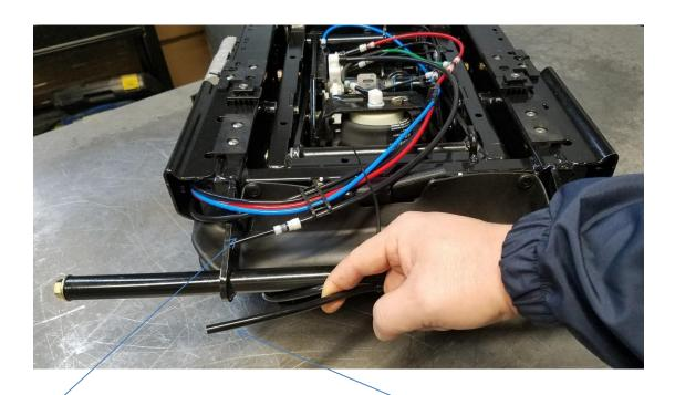
EXHAUST HOSE 1/8" VERY THIN HOSE DO NOT CONNECT! MUST BE OPENED! AIR IN HOSE
