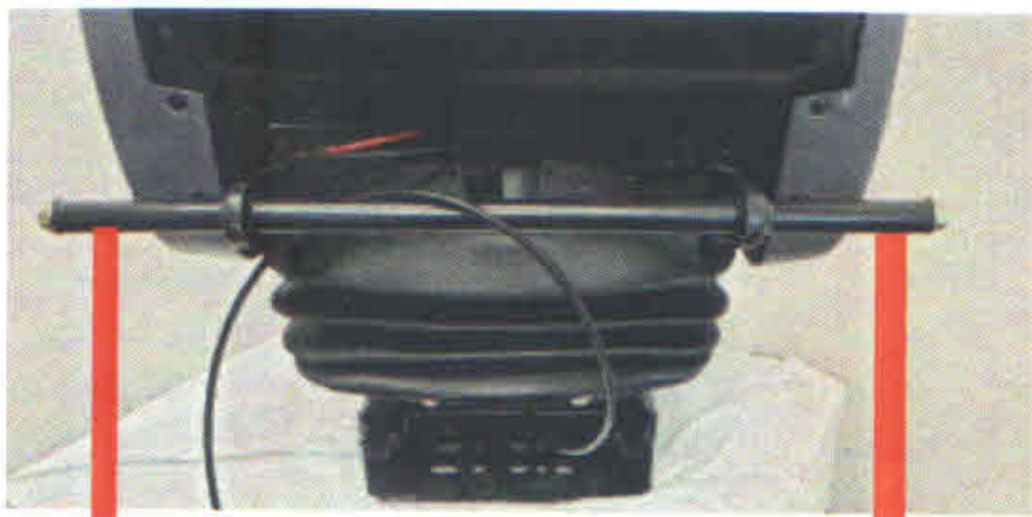
ICP/ Seat Belt Tethering bar(Bolts included) for your seat belt harness system(Except TC500 Series model)
