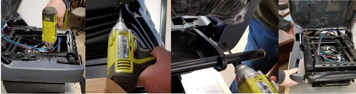
3<sup>rd</sup>, Locate VA005 into top of side bottom frame as you can see, use bolt and nuts for hold adaptor and use 2 small screws to guide both side of adaptor.
