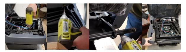
3<sup>rd</sup>, Locate VA005 into top of side bottom frame as you can see, use bolt and nuts for hold adaptor and use 2 small screws to guide both side of adaptor.
