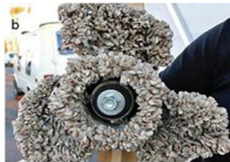
(b) Boat propeller encrusted with Dreissenid mussels
