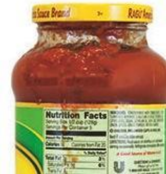
Signs of leakage
