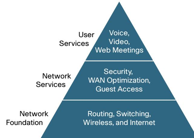
The Cisco Smart Business Architecture can be broken down into the following three primary, modular yet interdependent components for the midsize organization.
