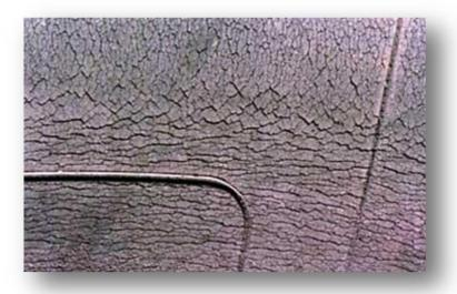
The surface cracks that occasionally appear have been called many things; Weather Checking, Weather Cracking or Ozone Cracking. These small cracks typically develop in the sidewalls or at the base of the tread grooves. Depending on their severity, they may be cosmetic in nature if they don't extend past the rubber's outer surface, or may be a reason to replace the tire if they reach deep into the rubber.
