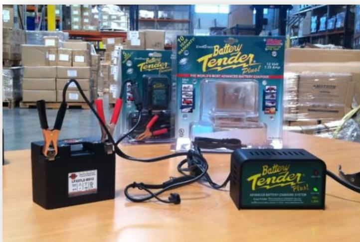
Charging is a process that reverses the electrochemical reaction. It converts the electrical energy of the charger into chemical energy. Remember, a battery does not store electricity; it stores the chemical energy necessary to produce electricity. (One example of a simple charger is shown in the picture)...you can get your charger at McDermott's HD and they can direct you to what is proper for your bike)!
