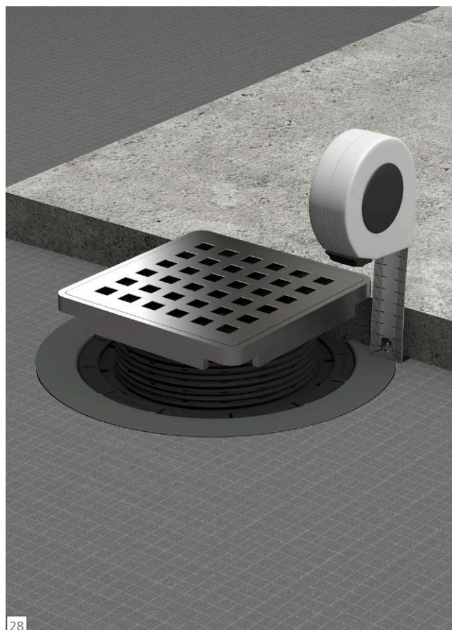
**EN** Dry-fit a tile for the shower base right next to the extended drain cover unit and determine to what height the Drain Cover Extension may need to be cut down for a drain cover top flush with the top of the tile (or drain cover top slightly below top of tile). Account for the thickness of the (compressed) thinset mortar used to install the tile. Using a ruler or measuring tape if necessary, match this measurement along the side of the Drain Extension piece.
