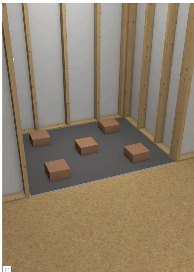
**EN** Press the Fundo firmly into the thinset bed (sloped side up) ensuring that the installation is level along its perimeter and sides, and thinset attachment and coverage is void free. Apply some weight equally and leave on surface and drain area to allow the thinset to initially cure without being disturbed (e.g. tile boxes). Make sure the floor waste pipe is centered within the wedi drain unit and remains there until the drain connection is completed.
