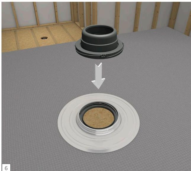
**EN** Insert the Drain Body snugly into the receiving mechanism of the Drain Unit on the underside of the Fundo base.
