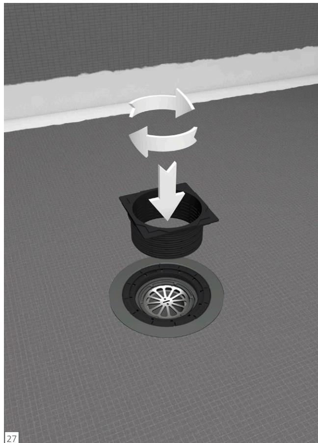
**EN** Next, insert the Drain Cover Extension into the threaded part of the Alignment Ring 1. Dry fit the Drain Cover Extension for the needed final height position of the drain cover unit. The Drain Cover Extension only works for wedi's finished surface drain covers, but not with wedi's tileable covers due to their special water drainage design. wedi Tileable covers are made to work with defined tile thicknesses and can be inserted into the Alignment Ring 1 and Snap Ring 2 assembly directly.
