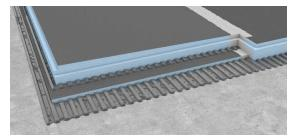
wedi shower bases thicker than 1 1/2 inches where an extension is connected require a wedi building panel be placed and thin-set mortar adhered under the extension panel to adjust for a proper connection fit.
