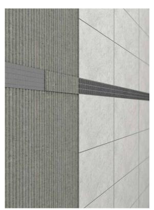
wedi's 1/8 inch Building Panel can be used to perfectly install mosaic accent strips into a large format wall tile assembly. This helps avoid excessive mortar build-up and leveling when trying to evenly align the field tile with the thinner mosaic tile strip. The strips of wedi Building Panel could even be pre-tiled in the shop and simply adhered into the wall assembly on-site using thinset mortar applied to the back of the strip only.
