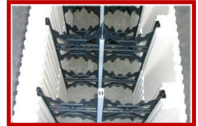
H Clip joining two 6" (15.2cm) spacers shown = 12.63" (32.07cm) concrete width
