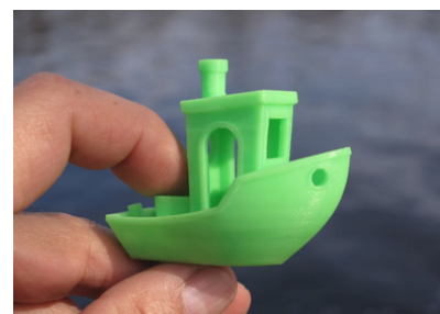
'Benchy' boat - a 3D benchmark test print
