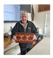
This board was created by cutting a series of accurate squares in Merbau and Mountain Ash. Coloured strips are the cut to suitable lengths and a number of steps are taken to glue the pieces together to create the Argyle pattern. After glueing, the board is cut to final size then with the outside edges rounded using the router the board is finally sanded and oiled.
