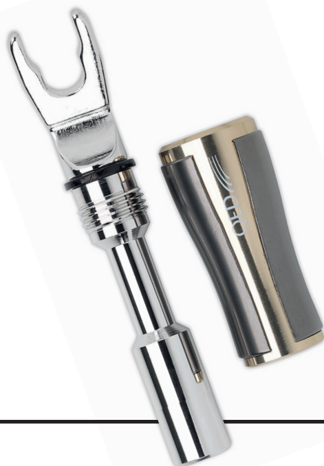
LEFT: Detail of QED's optional spade connector which is fashioned from a rhodium-plated high purity beryllium/copper and bonded to the cable with an 'Airloc cold weld' to exclude air
