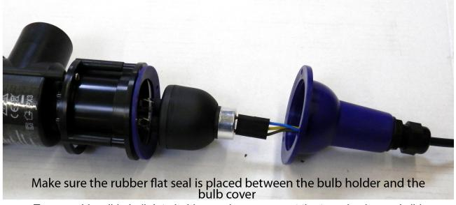
To assemble, slide bulb into holder as shown connect the two pin plug and slide the purple cap down the cable so that the three holes in the cap line up with the posts on the bulb holder and secure using the screws
