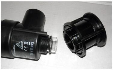
To clean the quartz tube, remove the bulb holder by firstly removing the bulb and undo the two retaining screws then unscrew (turn anti-clockwise) remove the o/ring, on a twin bulb unit both holders must be removed, the quartz can now be removed
