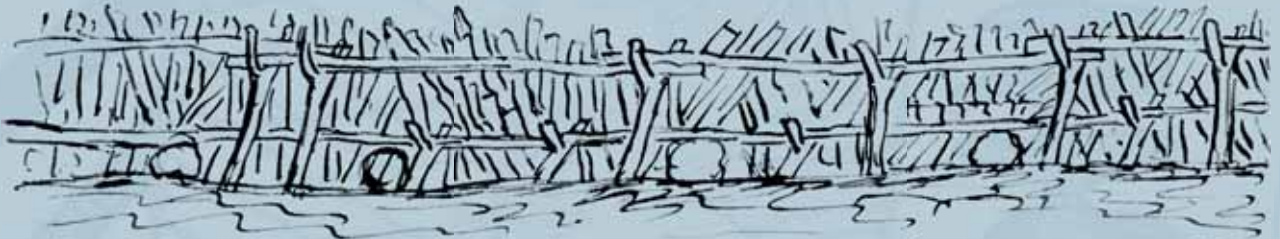
2.46 Detail of back of a large stake, branch and basket fishing weir, Moyne River (Robinson journal, 30 April 1841)
