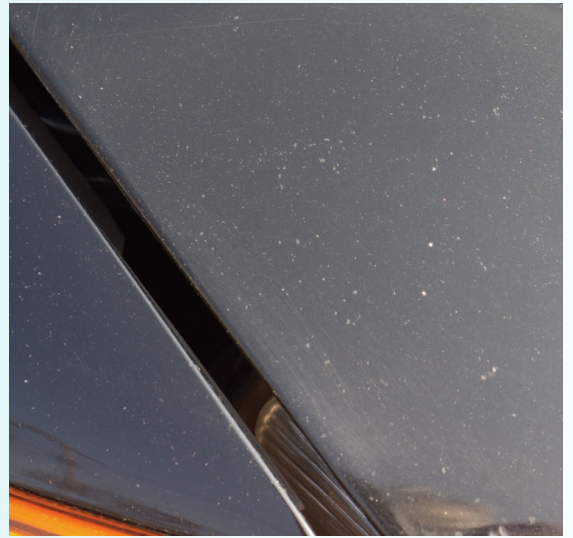
FIGURE 13—This image shows the longevity of a 1K UV-A primer and a 1K UV-A clearcoat after 8 years of service in the northeastern United States.
