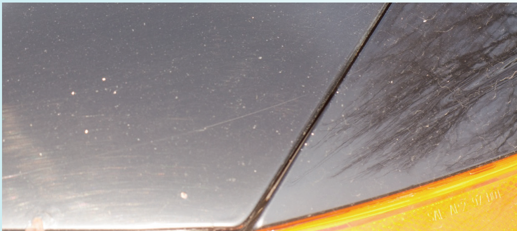
FIGURE 14—This image illustrates the longevity of a 2K PUR primer and clearcoat as the standard for comparing against the 1K UV-A primer and a 1K UV-A clearcoat after 8 years of service in the northeastern United States.
