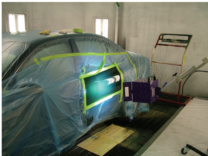
FIGURE 15—A 1K UV-A clearcoat has been introduced to the market, but it is currently difficult to find such products. Technical articles have been written on the 1K UV-A clearcoat technology and have shown some of the performance considerations that are needed to meet the automotive-refinish industry performance requirements.
