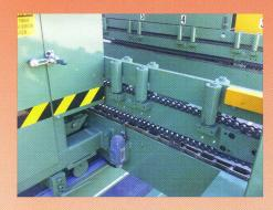
Heavy Duty Lumber Hold Downs provide positive, solid holding power for each piece. Each piece is held firmly in place during the initial trimming and the final cutting process.
