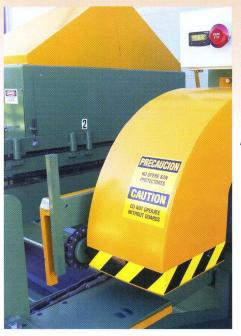
In addition to floor truss components, the FWA 500 will cut headers, window bucks, door bucks, soffit returns, bridging, fire blocks, and almost any type of double end 4x2 cutting up to 20ft. long.
