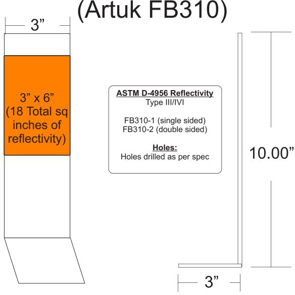
Our custom FB310 is made of high impact UV Stabilized ABS.125" thick. Perfect for any Top Mount Application
