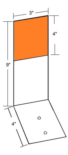
The marker body is made of high impact polycarbonate .090" (2.3mm) thick w/ (2) 1/4" mounting holes.
