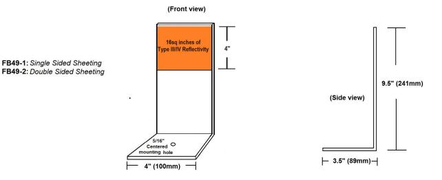
The FB49 is a top mount delineator that offers over **16** square inches of reflectivity. The marker body is made of a high impact polycarbonate .090" (2.3mm) thick and will flex instead of bend or break when struck. The combination of strength and visibility make this a great option for any top mount barrier application.
