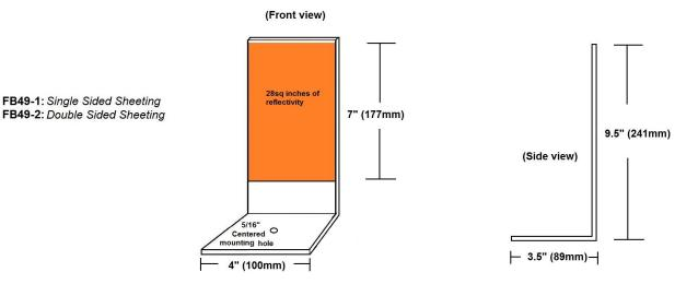
The FB49 is a top mount delineator that offers over 28 square inches of reflectivity. The marker body is made of a high impact polycarbonate .090" (2.3mm) thick and will flex instead of bend or break when struck. The combination of strength and visibilty make this a great option for any top mount barrier application.
