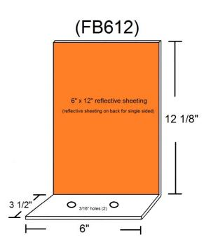
The Artuk FB53 (Side Mount) & FB612 (Top Mount) marker bodies are made of a high impact plastic 1/8" thickness.
