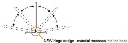
& body with added undercuts, further strengthening the bond (between hinge & body)
