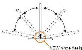
NEW hinge design - material recesses into the base & body with added undercuts, further strengthening the bond (between hinge & body)
