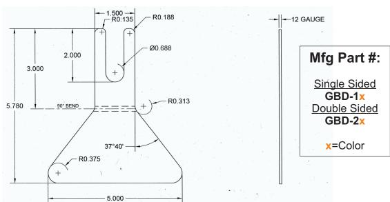
The Artuk Galvanized Bolt-On Delineator (GBD12) offers 8+ square inches of reflectivity, making it highly visible all season long (day or night). The marker body is made of Galvanized 12 Gauge Steel. Strong enough to withstand being hit repeatedly by snow plows and protecting it from any vandalism year after year.
