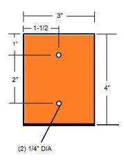
3" x 4" Delineator Plate w/ (2) 1/4" predrilled mounting holes and and 12sq inches of ASTM D4956 Type XI reflectivity
