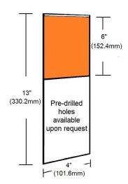
The bodies shall be made from a high-impact, weatherable engineering thermoplastic .090 (min) thick that conforms to the following:
