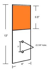
The bodies shall be made from a high-impact, weatherable engineering thermoplastic .090 (min) thick that conforms to the following:
