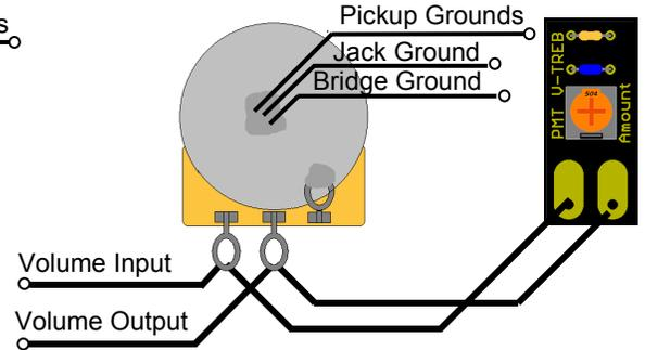
The V-Treb variable treble bleed/bypass circuit corrects the problem of high frequency losses at reduced volumes by allowing the player to control how bright or warm the tone will get as the volume control is reduced. With the volume at 10, the V-Treb is removed from the circuit and does not affect the sound.
