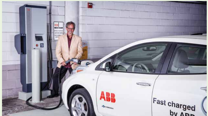
Ken Graber uses the newest DC charging station on campus to fully charge an EV in less than 90 minutes.
